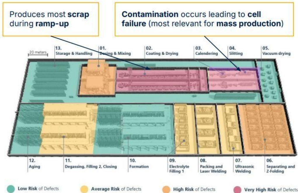
Figure 6 Layout of a typical, modular battery cell production line (7-10 GWh/a) and their risk level for defects. A battery cell factory has multiple of such modules/lines.
